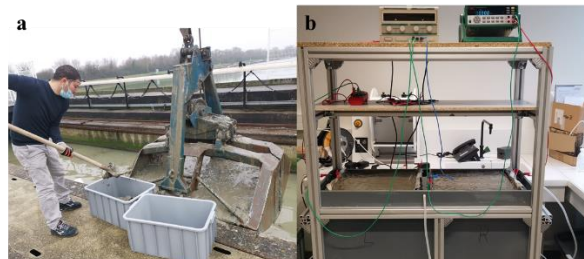
Collection of dredged sediments (a) and treatment using electrokinetics (b)
